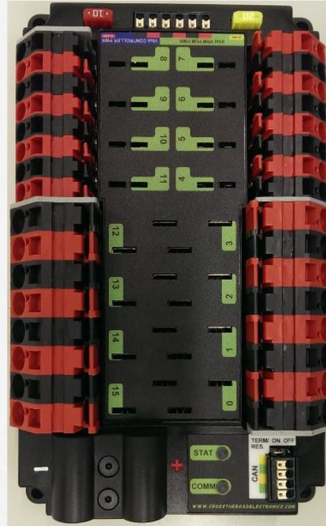
Power Distribution Panel (PDP)
